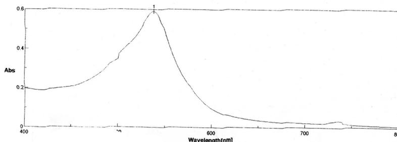
**Figure 2(a)-** UV Spectrum of CSWC at Normal pH ( $\lambda_{max}$  538nm)
